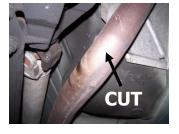
3. Then cut over axle tail pipe before axle and remove.
