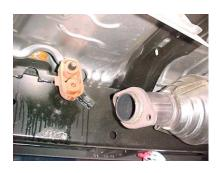
TO REMOVE STOCK EXHAUST UNBOLT IT FROM THE SLIP-FIT JOINT LOCATED IN THE REAR ABOVE THE AXLE AND SLIDE THE TAILPIPE OUT. NEXT UNBOLT THE 2-BOLT FLANGE LOCATED JUST BEHIND THE CATALYTIC CONVERTER. DO NOT THROW AWAY STOCK NUTS AND BOLTS YOU WILL NEED TO RE-USE THEM.
