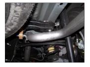
**5.** Next, install the exit pipe #D. Use clamp #F to secure to the tailpipe. DO NOT TIGHTEN. Insert welded hanger into rubber grommet.
