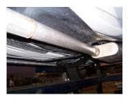
5. Install extension pipe #C onto muffler outlet. Use clamp #H to secure the pipe to the muffler. Insert welded hanger into rubber grommet.
