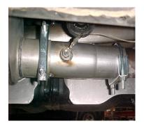
Install head pipe # A on to your existing stock front pipe and secure with clamp # F. Insert welded hanger into rubber grommet. Do not tighten. Install ground strap onto stud on your new head pipe. Use your factory nut.
