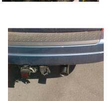
Install stainless tip. Clamp down. When you have everything in place, firmly tighten all bolts and clamp down securely. To clean stainless tip use any stainless cleaner and a scotch brite pad.
