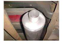
CONNECT MUFFLER #B TO THE FRONT EXTENSION PIPE WITH THE LOUVERS FACING TOWARDS THE CONVERTER. USE A JACK STAND TO SUPPORT THE MUFFLER AND CONNECT WITH CLAMP #E BUT DO NOT TIGHTEN. MUFFLER INLET IS LOOKING INTO THE LOUVERS.
