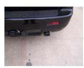
**8.** Install stainless steel tips. Clamp down. When you have everything in place, firmly tighten all bolts and clamps down securely. Use stainless steel cleaner and a Scotch Brite pad weekly to prevent tip from discoloration.
