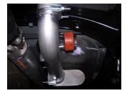
**6.** Install the intermediate tailpipe #C into the muffler  $1\frac{1}{2}$ "-2". Use clamp #G to secure tailpipe to muffler. DO NOT TIGHTEN.
