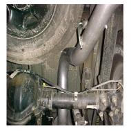
NEXT, INSTALL OVERAXLE TAILPIPE # D INTO MUFFLER 1-1/2"- 2". USE CLAMP # I TO SECURE PIPE TO MUFFLER, DO NOT TIGHTEN.
