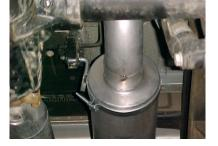
NEXT, INSTALL BAND CLAMP # H ONTO MUFFLER INSERT HANGER INTO RUBBER GROMMET. USE BOLT KIT PROVIDED FOR BAND CLAMP, DO NOT TIGHTEN.
