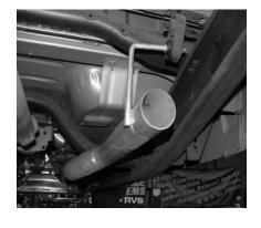
BOLT HEADPIPE #A TO THE STOCK FLANGE RE-USING THE FACTORY NUTS & BOLTS. INSERT WELDED HANGER INTO RUBBER GROMMET. DO NOT TIGHTEN.
