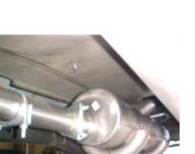
Install muffler # B onto head pipe 1-1/2" to 2" with the louvers facing towards the converter. Use a jack stand to support the muffler. Use clamp #E to secure the muffler to the head pipe. Do not tighten. Muffler inlet is looking into the louvers. Outlet should be at 10 o'clock position.
