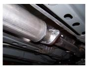
3. Install resonator #A on to vour existing 2-bolt flange and secure with bolt kit #E. Do not tighten. Use a jackstand to support the resonator.
