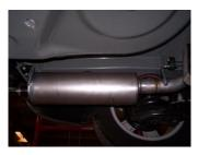
6. Slide muffler #D onto overaxle pipe and insert welded hanger into rubber grommet. Use clamp #F to secure muffler to overaxle pipe.
