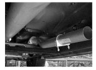
INSTALL MUFFLER # B ONTO HEADPIPE  $1\frac{1}{2}$ " TO 2" WITH INLET TOWARDS THE MOTOR MUFFLER INLET IS LOOKING INTO THE LOUVERS. MUFFLER OUTLET SHOULD BE AT THE 8 O'CLOCK POSITION.
