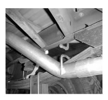
INSTALL THE OVERAXLE TAILPIPE #C INTO MUFFLER AT LEAST 1 1/2" TO 2" USING CLAMP #G. DO NOT TIGHTEN. INSERT WELDED HANGERS INTO RUBBER GROMMETS. THE SPARE TIRE ON SOME VEHICLES MAY NEED TO BE LOOSEN AND PULLED TO THE DRIVER SIDE AND **RE-TIGHTENED.** ROTATE PIPES UNTIL YOU HAVE AT LEAST A 1" CLEARANCE AWAY FROM SHOCK, BRAKE LINES, SPARE TIRE ECT.
