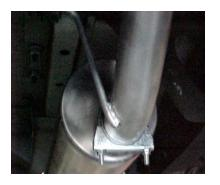
SLIDE MUFFLER WITH DUAL INLET ONTO HEADPIPE AT LEAST 1-1/2" TO 2". MUFFLER OUTLET SHOULD BE AT THE 6 O'CLOCK POSITION. USE CLAMPS #F TO ATTACH IT TO THE HEADPIPE. INSERT WELDED HANGER INTO RUBBER GROMMET. MAKE SURE INLETS AND MUFFLER IS LEVEL. AND TIGHTEN DOWN. USE JACK STAND TO SUPPORT MUFFLER.
