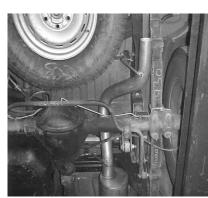
INSTALL THE OVERAXLE TAILPIPE #C INTO MUFFLER AT LEAST 1 1/2" TO 2" USING CLAMP #G. DO NOT TIGHTEN. INSERT WELDED HANGERS INTO RUBBER GROMMETS. THE SPARE TIRE ON SOME VEHICLES MAY NEED TO BE LOOSEN ED AND PULLED TO THE DRIVER SIDE AND **RE-TIGHTENED.** ROTATE PIPES UNTIL YOU HAVE AT LEAST A 1" CLEARANCE AWAY FROM ALL PIPES, ETC.
