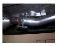
2. To remove the stock exhaust, unbolt the 2 bolt flange located in front of the new muffler. Disengage the welded hangers using WD-40 from the OEM rubber grommets. Do not damage or remove the rubber grommets as you will reuse them to mount your new system. Now, cut off tailpipe and remove exhaust.
