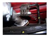
3. Install headpipe #A onto your existing stock flange using bolt kit #F to secure flange. DO NOT TIGHTEN. Insert welded hanger into rubber grommet.
