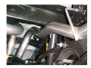
7. Slide the passenger side tailpipe #E into muffler 1.5-2". Insert welded hanger into rubber grommet. Use clamp #G to secure tailpipe to muffler. DO NOT TIGHTEN.
