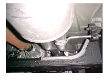
Install muffler #C onto head pipes B 1-1/2" to 2" with the louvers facing towards the converter. Use a jack stand to support the muffler. Use clamps #G to secure the muffler to the head pipes. Do not tighten. Outlet of muffler should be at 6 o'clock.
