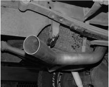
INSTALL TURNOUT PIPE # D ONTO OVERAXLE TAILPIPE USING CLAMP # E. INSERT WELDED HANGER INTO RUBBER GROMMET. DO NOT TIGHTEN.
