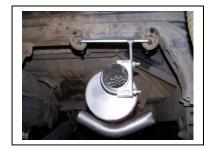
Install muffler # B onto head pipe # A 1-1/2" to 2" with the louvers facing towards the converter. Use a jack stand to support the muffler. Use clamp #F to secure the muffler to the head pipe. Do not tighten. Muffler inlet is looking into the louvers.
