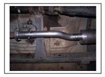
Attach head pipe # A on to your existing stock front pipe and secure with bolt kit # E. Use a jack stand to support the converter. Insert welded hanger into rubber grommet. Do not tighten.
