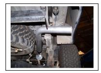
Install stainless steel tip. Clamp down. When you have everything in place, firmly tighten all bolts and clamps down securely. To clean stainless steel tip use any stainless steel cleaner and Scotch Brite pad.
