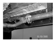
2. To remove the stock exhaust, unbolt it at the 2-bolt flange located in front of the muffler. Disengage hangers from OEM rubber grommets. Use WD-40 to aid in this process. Do not damage or remove the OEM rubber grommet as you will reuse them to mount your new system.
