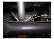
5. Slide the over axle tailpipe #C into the muffler  $1\frac{1}{2}$ "-2". Insert welded hangers into rubber grommets. Use clamp #E to secure the muffler and tailpipe together. Do not tighten.
