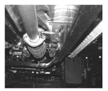
BOLT HEADPIPE #A TO STOCK FLANGE. RE-INSTALL O2 SENSOR USING FACTORY GASKET, INTO HEADPIPE BEHIND FLANGE AND USE BOLT KIT #G TO ATTACH. WE RECOMMEND TO USE O2 SENSOR SAFE GASKET SEALER TO HELP PREVENT LEAKS.
