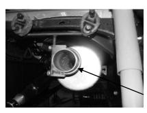
INSTALL REAR MUFFLER HANGER #F AT THE REAR OF THE MUFFLER AND ATTACH TO RUBBER GROMMETS. THE VERTICAL ROD WILL BE AIMING UP ON THE DRIVER SIDE OF THE VEHICLE.
