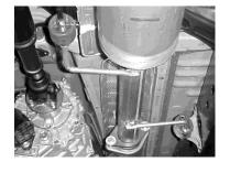
Install head pipe # A on to your existing stock 2 bolt flange. Use hardware kit #G, to secure. DO NOT TIGHTEN.
