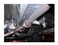
Lay out the exhaust on the floor so it looks like the drawing and compare parts with manual. To remove the stock exhaust remove, it from the 2-bolt flange, just in front of the muffler. Then cut your tailpipe off behind your factory
