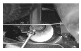
INSTALL OVERAXLE TAILPIPE # C INTO THE MUFFLER, USING CLAMP # E. INSERT WELDED HANGER INTO RUBBER GROMMET.
