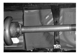
SLIDE THE HEADPIPE ONTO THE STOCK HEADPIPE USING CLAMP # E. THEN INSTALL THE MUFFLER ON HEADPIPE #A NO LESS THAN 1-1/2" TO 2" USING CLAMP #E. THE MUFFLER OUTLET WILL BE CLOCKED AT 12 O'CLOCK POSITION. INLET OF MUFFLER HAS LOUVERS FACING THE MOTOR. DO NOT TIGHTEN
