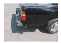
Install stainless steel tip. Clamp down. When you have everything in place, firmly tighten all bolts and clamp down securely. To clean stainless steel tip use any stainless steel cleaner and Scotch Brite pad.
