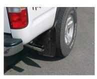
INSTALL THE STAINLESS TIP. USE A STAINLESS STEEL OR ALUMINUM CLEANER AND ANY SCOTCH BRITE PAD TO CLEAN. NOW TIGHTEN ALL HANGERS AND CLAMPS.
