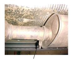
FOR EASIER REMOVAL OF THE FACTORY EXHAUST. CUT THE TAILPIPE BEHIND THE MUFFLER. THEN REMOVE THE FACTORY MUFFLER AT THE CLAMP IN FRONT OF THE MUFFLER. USE A JACK STAND TO SUPPORT THE CONVERTER ONCE EXHAUST IS REMOVED. NOTE LEAVE ALL FACTORY RUBBER GROMMETS IN PLACE
