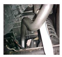
TAILPIPE #B INTO THE MUFFLER 1 ½" TO 2". SECURE TO THE MUFFLER USING CLAMP #D. DO NOT TIGHTEN. INSERT WELDED HANGERS INTO RUBBER GROMMETS. NOTE, SHORT END OF OVER AXLE PIPE INSERTS INTO MUFFLER.
