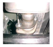
ATTACH MUFFLER ASSEMBLY #A ONTO YOUR EXISTING STOCK FLANGE. USE BOLT KIT # E TO SECURE TO FLANGE. USE A JACK STAND TO SUPPORT THE MUFFLER.
