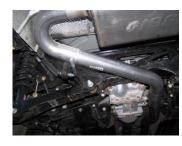
5. Slide inlet pipe #C over the intermediate pipe. Insert welded hanger into rubber grommet. Secure with clamp #G. Do not tighten.
