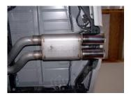
7. Install rear muffler assembly #F onto tailpipes. Use clamps #G to attach muffler to tailpipes. Do not tighten. Insert welded hangers into rubber grommets.
