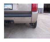
6. Install stainless steel tips. Clamp down. When you have everything in place, firmly tighten all bolts and clamps down securely. Use stainless steel cleaner and a Scotch Brite pad weekly to prevent tip from discoloration. Inspect all fasteners after 25-50 miles of operation and re-tighten as necessary
