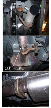
1. To remove the stock exhaust remove the nut on the rear hanger using a 21mm wrench, then cut the tailpipe just after the rear muffler hanger and remove. Unbolt the headpipe at the flange and remove. Leave all rubber grommets in place. Use WD-40 to aid in removal of hangers from rubber grommets.
