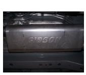
3. Install muffler #B onto headpipe #A 11/2-2" with the louvers facing towards the converter. Use a jack stand to support the muffler. Use clamp #F to secure the muffler to the headpipe. DO NOT TIGHTEN.
