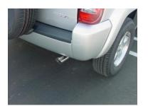
INSTALL THE STAINLESS STEEL TIP. TO CLEAN TIP USE A SCOTCH BRITE PAD AND ANY STAINLESS OR ALUMINUM CLEANER. NOW GO BACK AND TIGHTEN ALL CLAMPS, NUTS AND BOLTS STARTING FROM THE FRONT AND WORKING BACK.
