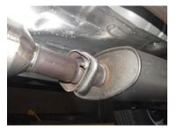
REMOVE STOCK EXHAUST UNBOLT THE STOCK FLANGE LOCATED JUST BEHIND THE CATALYTIC CONVERTER. LEAVE ALL RUBBER GROMMETS IN PLACE. USE WD-40 TO AID IN THE REMOVAL OF EXHAUST AND HANGERS.
