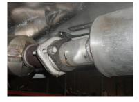
INSTALL FLANGE #B ONTO THE HEADPIPE #A. USE BOLT KIT #G TO SECURE HEADPIPE #A TO STOCK FLANGE. DO NOT TIGHTEN.
