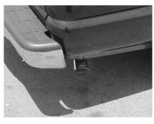
4. BEFORE INSTALLING OVERAXLE TAILPIPE. YOU MUST UNBOLT FACTORY REAR TAILPIPE HANGER AND ROTATE IT 180 **DEGREES**. Insert the overaxle tailpipe. #C no less than  $1\frac{1}{2}$  and no more than 2". Slightly lean to the driver side. Slide turnout pipe #D on to the tailpipe. Roll turnout pipe until you have it at the correct angle for your truck. Insert welded hanger into rubber grommet. Clamp down. Using clamp #G
