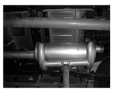
1. Lay out the GIBSON EXHAUST SYSTEM on the floor so it looks like the drawing. Match all part numbers with the manual. Un-bolt the stock exhaust from the 3-bolt flange located behind the catalytic converter. Leave all rubber grommets in place. Use jack stands to support converter.
