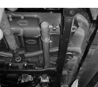
2. Bolt on front headpipe #A using bolt kit #I and gasket #H. Use a RTV gasket sealer for flange connection. (Note Headpipe will lean toward passenger side.)
