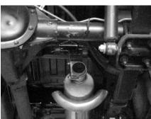
3. Slide muffler #B no less than  $1\frac{1}{2}$  and no more than 2" onto the front headpipe with louvers in muffler facing towards the converter. Use a jack stand to support the muffler. Outlet of muffler should be clocked at 9 o'clock. Attach using clamp #G. Install rear hanger #F onto muffler. Do not tighten. Muffler inlet is looking into the louvers.
