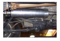
**INSTALL MUFFLER #B** ONTO HEADPIPE #A WITH **INLET TOWARDS THE** MOTOR. INLET OF MUFFLER IS LOOKING INTO THE LOUVERS USE CLAMP #E TO SECURE MUFFLER TO THE HEADPIPE, DO NOT TIGHTEN. OUTLET OF MUFFLER SHOULD BE AT THE 10 O'CLOCK POSITION.
