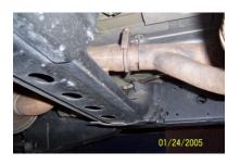
TO REMOVE STOCK EXHAUST, REMOVE IT FROM THE CLAMP LOCATED IN FRONT OF YOUR STOCK MUFFLER. **NEXT REMOVE THE FACTORY 12 MM NUT ON** THE REAR TAILPIPE. DO NOT DISCARD YOU WILL REUSE IT.
