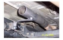
**INSTALL HEADPIPE #A** ONTO STOCK PIPE, USE CLAMP# E TO SECURE PIPES TOGETHER. DO NOT TIGHTEN. NEXT, MOUNT WELDED HANGER TO RUBBER **GROMMET USING BOLT** KIT # F.
