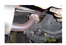
LAY OUT THE GIBSON EXHAUST ON THE FLOOR AND COMPARE PART #'S TO THE DRAWING. TO REMOVE YOUR FACTORY EXHAUST UN-BOLT YOUR TAILPIPE AT THE 2-BOLT FLANGE LOCATED BEHIND YOUR STOCK MUFFLER USE WD-40 TO AID YOU IN REMOVAL OF HANGERS FROM RUBBER GROMMETS.
