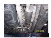
RESONATOR 1 1/2" -2". USE CLAMP # G TO SECURE MUFFLER TO THE PIPE, DO NOT TIGHTEN. MUFFLER **OUTLET SHOULD BE** AT THE 10 O'CLOCK POSITION. REMOVING THE SPARE TIRE WILL MAKE FOR EASIER **INSTALLATION OF** TAILPIPE.. AFTER YOUR DONE REINSTALL THE SPARE TIRE.
