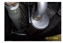
INSTALL BAND CLAMP # F ONTO MUFFLER, INSERT HANGER INTO RUBBER GROMMET, USE BOLT KIT PROVIDED, DO NOT TIGHTEN.
