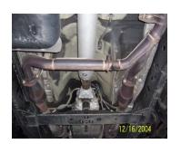
NEXT, UN-BOLT YOUR EXHAUST FROM THE 2-BOLT FLANGES LOCATED JUST BEHIND YOUR FACTORY CATALYTIC CONVERTERS, DO NOT DISGUARD YOUR FACTORY GASKETS AND HARDWARE YOU WILL RE-USE IT.
