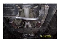
INSTALL Y-PIPE # A & I ONTO STOCK FLANGES USE YOUR STOCK HARDWARE TO SECURE. INSERT WELDED HANGER INTO RUBBER GROMMET, DO NOT TIGHTEN.
