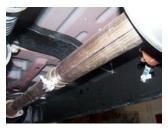
TO REMOVE YOUR STOCK EXHAUST, REMOVE IT FROM FLANGE LOCATED JUST IN FRONT OF THE MUFFLER REMOVE HANGERS FROM RUBBER GROMMETS BY PULLING EXHAUST TOWARDS THE REAR OF THE VEHICLE, USE WD-40 TO AID IN REMOVAL, LEAVE GROMMETS IN PLACE.
