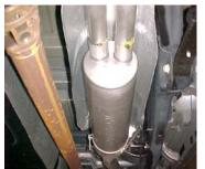
INSTALL MUFFLER # B ONTO HEADPIPE 1  $\frac{1}{2}$ " TO 2". USE CLAMP # G TO SECURE MUFFLER TO HEADPIPE. DO NOT TIGHTEN. USE A JACK STAND TO HOLD UP THE MUFFLER. OUTLETS SHOULD BE LEVEL.
