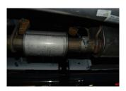
1. To remove the stock exhaust remove it from the clamp located behind the stock resonator. Disengage the welded hangers using WD-40 from the OEM rubber grommets. Do not damage or remove the rubber grommets as you will re-use them to mount your new system. Now, cut off tailbipe and remove exhaust.
