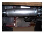
3. Install muffler #B onto head pipe #A 1½"-2" with the louvers facing towards the converter. Muffler outlets should sit level. Use a jack stand to support the muffler. Use clamp #G to secure the muffler to the headpipe. Do not tighten.
