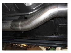
2.Install headpipe #A onto your factory pipe using clamp #G insert welded hanger into the rubber grommet leave clamp loose.
