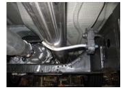
Bolt head pipe #A to the Factory pipe. Insert welded hanger into rubber grommet. Do not tighten.
