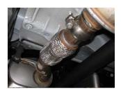
2. To remove stock exhaust, the Y-pipe. Make sure to leave all rubber grommets in the factory location. You will reuse stock clamp. For easier removal of exhaust, cut behind the muffler. Use WD-40 to remove hangers from grommets.
