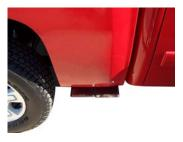
5. Install right and left stainless steel tips. Clamp down. When you have everything in place, firmly tighten all bolts and clamps down securely. Use stainless steel cleaner and a Scotch Brite pad weekly to prevent tip from discoloration. Inspect all fasteners after 25-50 miles of operation and retighten as necessary.
