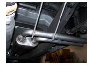
4. Rotate the muffler assembly until the outlets are level.
