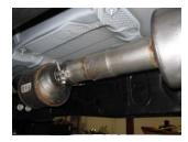
3. Install the muffler assembly onto the factory dome 2". Use a jack stand to support the muffler assembly. Use your factory clamp to secure muffler assembly to the dome. Do not tighten. Insert welded hangers into rubber grommets.
