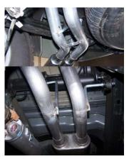
6. Now install driver side tailpipe #D. The spare tire may need to be loosened and pushed to the driver side to allow for clearance. Use bolt kit #H to attach both tailpipes together.
