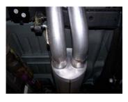
4. Install muffler #B onto headpipe 1.5-2" with the louvers facing towards the converter. Use a jack stand to support the muffler. Use clamp #G to secure the muffler to the headpipe. Do not tighten. Muffler inlet is looking into louvers.
