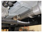
3. Install headpipe #A onto your existing stock flange and attach using stock hardware. Do not tighten. Insert welded hanger into rubber grommet.
