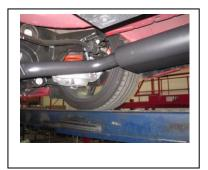
3. Now install the passenger side tailpipe assembly #B by sliding the metal hangers into the rubber grommets. Use clamp #D to secure together.
