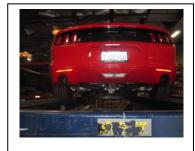
5. When you have everything in Place, firmly tighten all bolts And clamps down securely Use stainless steel cleaner and weekly to prevent tip from discoloration.
