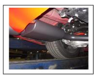
4. Now do the same procedure for the driver side. Use clamp # D to secure to the muffler.
