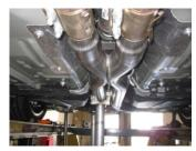
2. Install your Gibson x-pipe using the stock clamps
