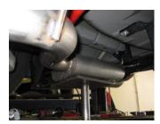
3. Now install the passenger side muffler assembly #B by sliding the metal hangers into the rubber grommets. Then do the same for the driver side muffler assembly #A. Use clamp #D to secure together.
