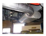
4. Now do the same procedure for the driver side. Use clamp # D to secure to the muffler.
