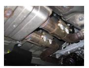
1. To remove your stock exhaust, unbolt it from the clamps located just after the manifolds then remove the whole exhaust system
