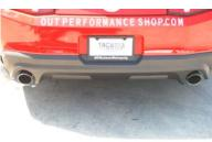
5. When you have everything in Place, firmly tighten all bolts And clamps down securely Use stainless steel cleaner and Scotch Brite pad weekly to prevent tip from discoloration. Inspect all fasteners after 25-50 miles of operation and re-Tighten as necessary
