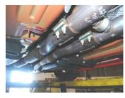
2. Loosen up the 2 clamps in the middle of the vehicle and slide them over the tailpipes. Now separate both tailpipes from mufflers and slide them out. Next remove the stock mufflers by sliding them out of the stock rubber grommets.
