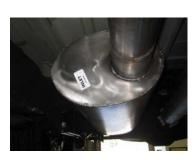
5. Install muffler #B onto head pipe #A 1½"-2" with the louvers facing towards the converter. Use a jack stand to support the muffler. Use clamp #e to secure the muffler to the head pipe. Muffler outlet position will be about 3:00. Do not tighten. Muffler inlet is looking into the louvers.
