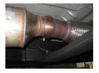
2. Remove your stock tail pipe from stock muffler by cutting it off just behind the stock muffler use wd-40 to help in removal of the hangers from the rubber grommets. Leave all rubber grommets on the factory hangers and on the vehicle.
