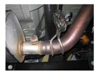
3. Remove the rest of your stock exhaust from the clamp located in front of your stock muffler.
