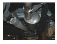
4. Install muffler #B onto headpipe  $1\frac{1}{2}$ "-2" with the louvers facing towards the converter. Muffler outlet will be at the 9 o'clock position. Use a jack stand to support the
