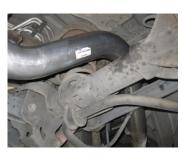
**5.** Install tailpipe #C into muffler 1½-2" and secure with clamp #F. DO NOT TIGHTEN. Insert welded hanger into rubber grommet.
