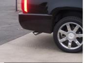
**7.** Install stainless steel tip #E. Clamp down. When you have everything in place, firmly tighten all bolts and clamps down securely. Use stainless steel cleaner and a Scotch Brite pad weekly to prevent tip from discoloration.
