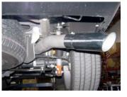
7. Install exit pipe #D into the tailpipe 1½-2" and secure with clamp #F. DO NOT TIGHTEN. Rotate pipe to best suit your vehicle.
