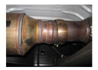
2. To remove the stock exhaust, unbolt it at the 2-bolt flange located in front of the muffler. Disengage the welded hangers using WD-40 from the OEM rubber grommets. Do not damage stock nuts and bolts or remove the rubber grommets as you will re-use them to mount your new system. Now, cut off tailpipe and remove exhaust.
