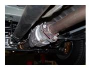
1. To remove the stock exhaust remove it from the 3-bolt flange located in front of the muffler. Disengage the welded hangers using WD-40 from the OEM rubber grommets. Do not damage factory hardware or remove the rubber grommets as you will re-use them to mount your new system.
